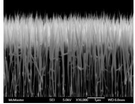
Nanowire Solar Cell: The nanowires create a surface that is able to absorb more sunlight than a flat surface – McMaster Univ., 2008
