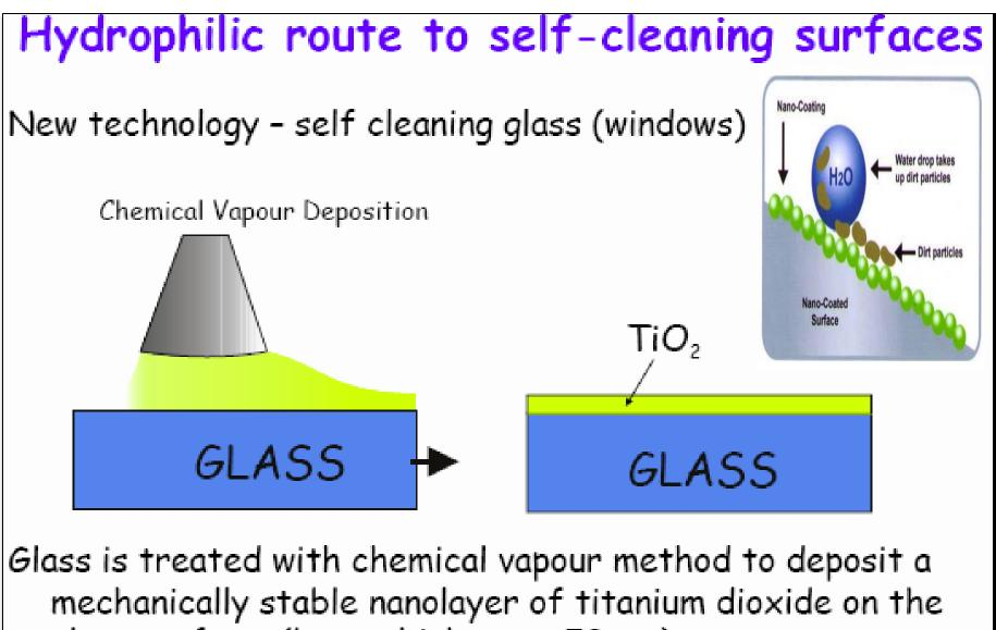
glass surface. (layer thickness ~50 nm)
