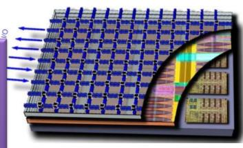
A silicon processor featuring on-chip nanophotonic network – *IBM Corp., 2008*
