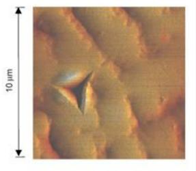
With a Nano-Indentation Tester you can quickly determine properties such as hardness and Young's modulus on almost any type of material - soft, hard, brittle or ductile.
