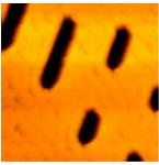
Number of pits = 4 (approximetly) Width of pits = 0.442 to 0.539 micror um 0.39 Length of pits = 1.20 to 2.38 micron 0.20-Depth of pits = 0.2 micron 0.00 Seperation between two pits: horizontally = 1.25 to 1.43 r vertically = 1.36 micron Scan size = 5 micron
