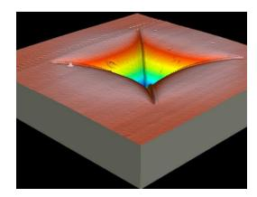
Nano-Indentation Tester is a high precision instrument for the determination of the nano mechanical properties of thin films, coatings and substrates.
