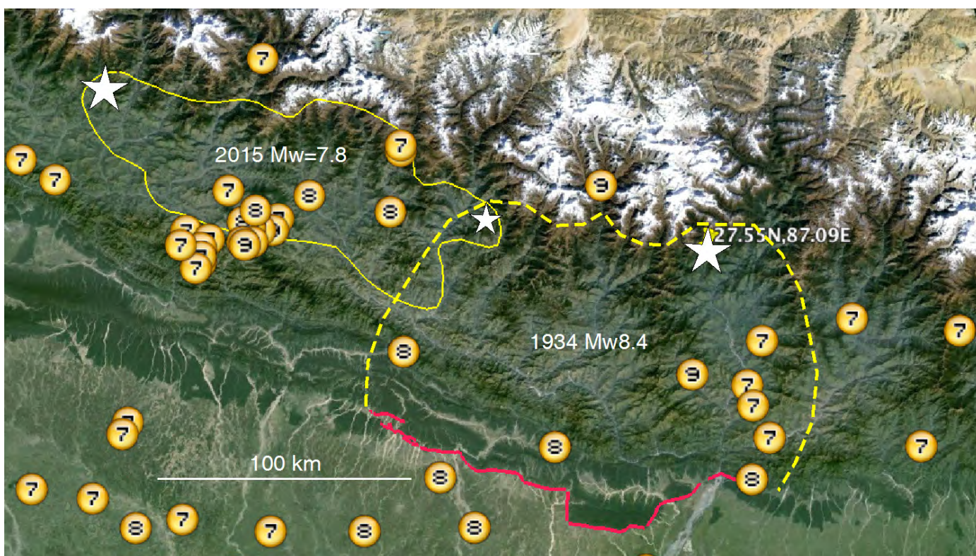
Figure 7 Reported EMS intensities for the Nepal 1934 M_w=8.4 earthquake (Martin and Szeliga, 2004) with a conjectural rupture zone (dashed). Epicenter is from Chen and Molnar (1987) and MFT rupture from Sapkota et al., 2012. Intensities above the 1934 rupture are sparse but average EMS\ 7.6 \pm 0.7 . With the conjectural rupture shown, mean slip in 1934 would be \approx 8\text{ m} .
